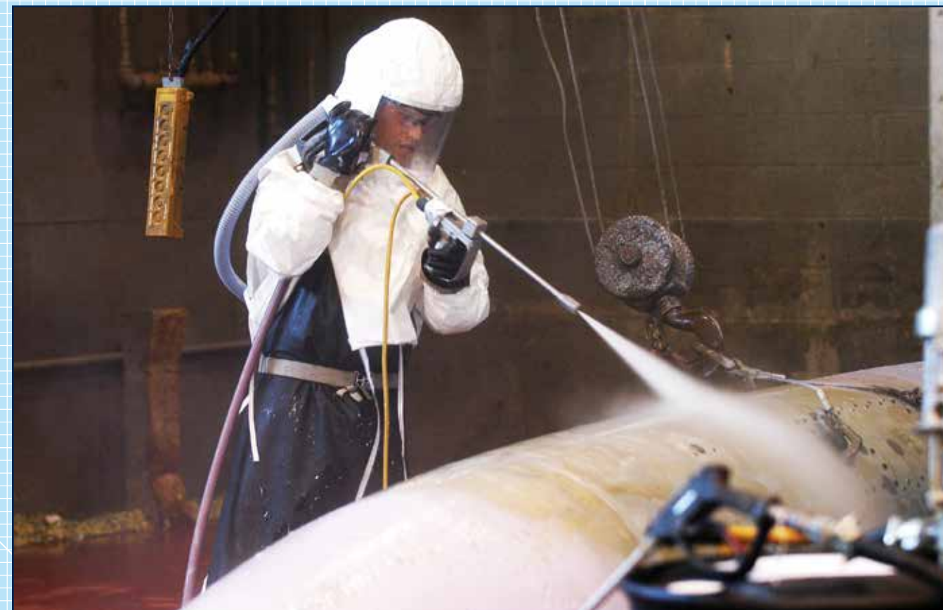
Kyle Jackson uses an Aqua Miser to remove paint from an F-15 fuel tank at Robins AFB, Georgia. New improvements to the HVAC system will improve working conditions in the area. The Air Force uses a rigorous chemical authorization and tracking process that enables compliance with laws, regulations and reporting requirements for hazardous chemicals. (U.S. Air Force photo/Sue Sapp)
