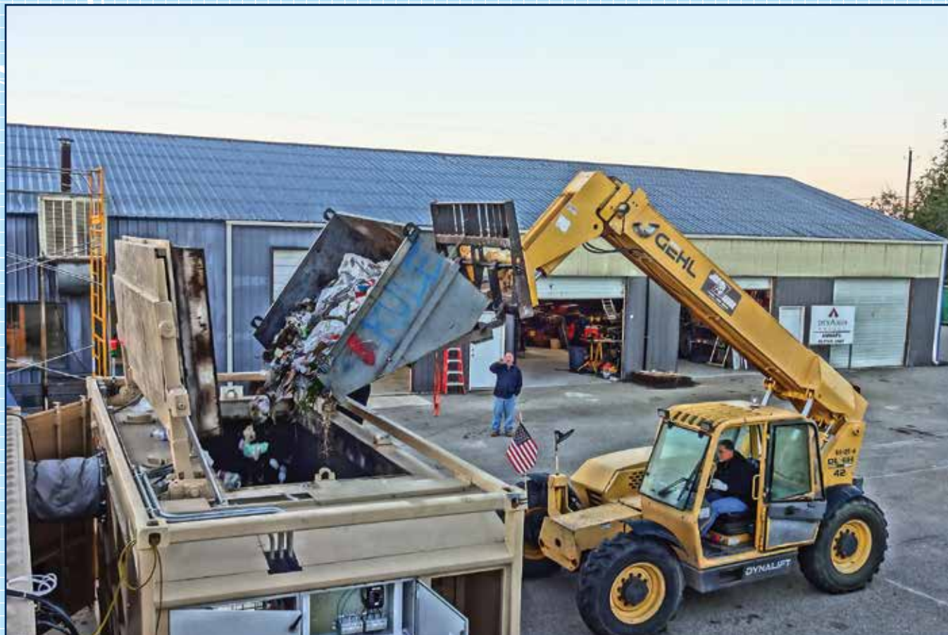
A waste-to-energy, large-scale gasification system prototype is energy efficient and eliminates hazardous emissions associated with open-pit burning. (U.S. Air Force photo/Mekka Parish)
