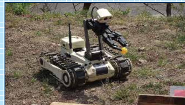
A small, 'back packable' robot has been developed for use by explosive ordnance disposal teams. (Courtesy photo)
