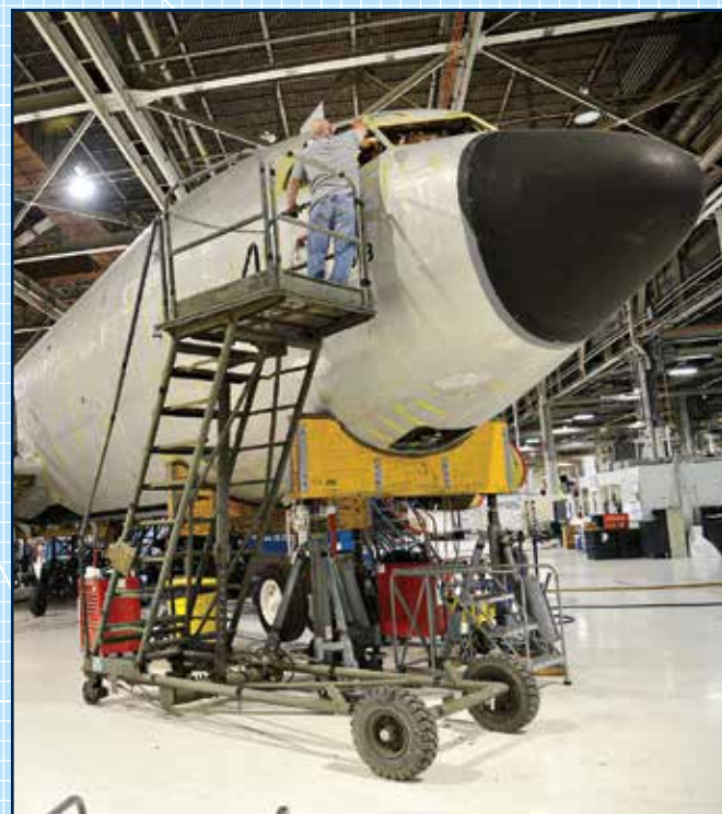
Aircraft Mechanic Steven Harris, 564th Aircraft Maintenance Squadron, preps window areas for installation on a KC-135 Stratotanker at the Oklahoma City Air Logistics Complex at Tinker Air Force Base, Oklahoma. The energy-saving performance contract awarded to Honeywell International Inc. at Tinker will include process energy conservation measures at the OC-ALC to reduce energy usage. (U.S. Air Force photo/Kelly White)
